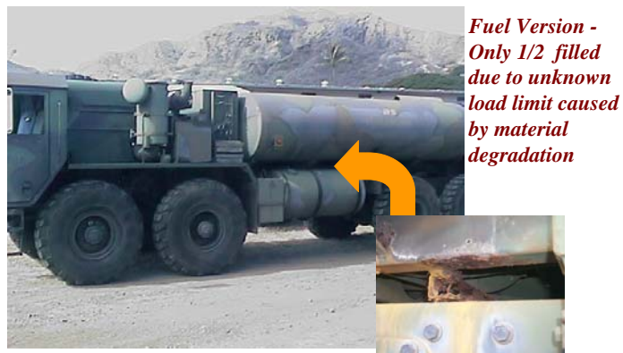
Figure 3. Fuel version of HEMTT with corroded supports
