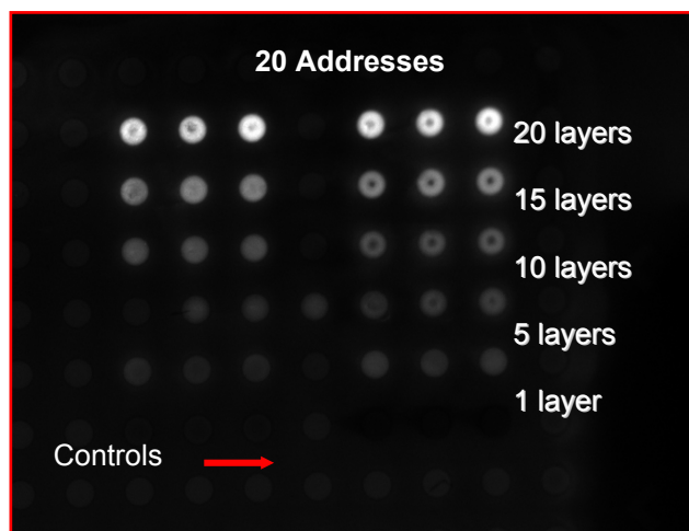
Figure 4 - Experiment showing one, five, ten, fifteen and twenty addressing with biotin and streptavidin quantum dots.
