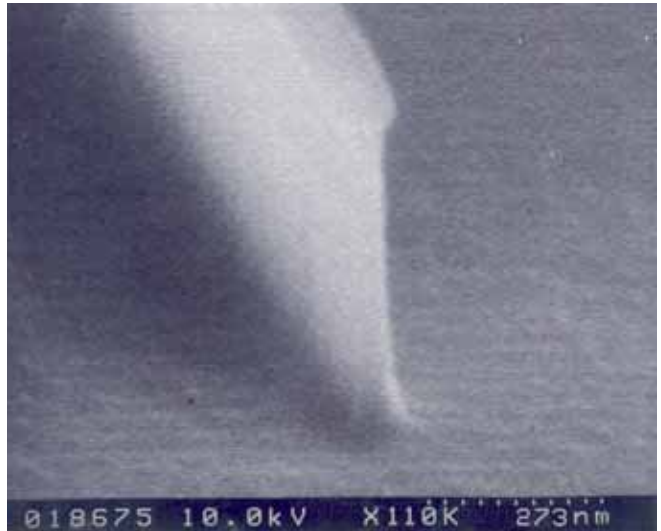
Figure 3: SEM micrograph of 90nm isolated resist line on silicon, with 21:1 aspect ratio, formed in 1.89\mu\text{m} thick OIR-89 resist using the 2-step NERIME process. The wafer received a \text{Ga}^+ beam exposure dose of 1.15 \times 10^{-2} \text{ C/cm}^2 , and was dry developed for 1350s in an \text{O}_2 plasma etch at 2mTorr pressure.
