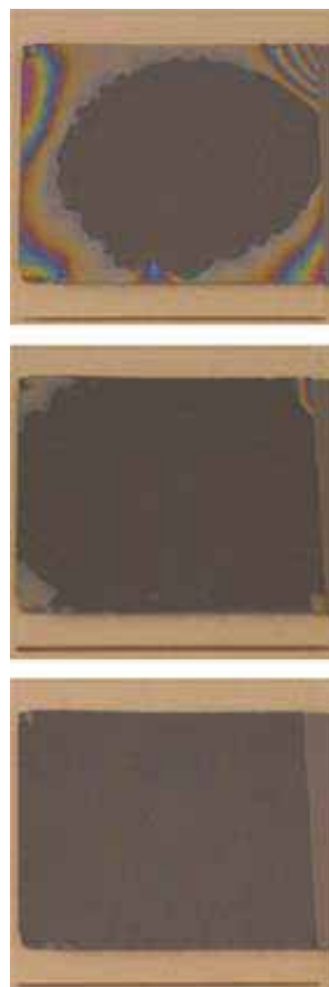
Figure 3. Still photos show resist spreading with time. Interference fringes spread out and disappear with time after contact between the mold and substrate: (a) 2 min; (b) 5 min; (c) 30 min.
