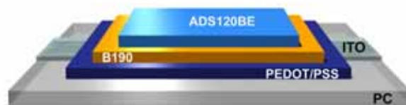
Figure 7: Setup of a multilayer system used for OLEDs
