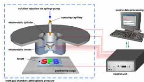
Figure 1: Experimental Setup of Atmospheric-Pressure Ion Deposition
