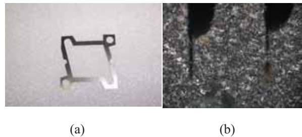
Figure 3. The shapes of filler metal sheets and cross section at each brazing case. (a) nickel foil, thickness: 38μm, width 3.5mm (b) Cross section of brazed stack (×100)
