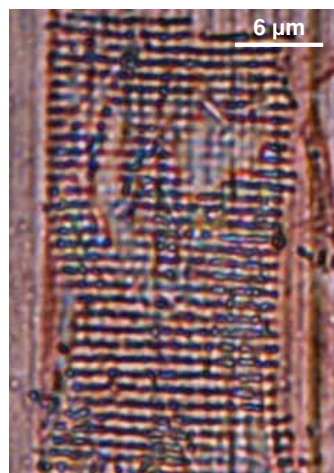
Figure 2: Sub-micron photo-patterned features in the organic-inorganic hybrid material on a Cu substrate.
