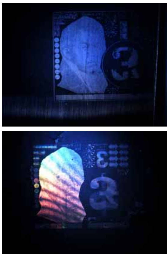
Figure 1: Diffractive OVD photo-patterned into organic-inorganic hybrid material on Cu substrate, as viewed with two different angles of white light illumination.
