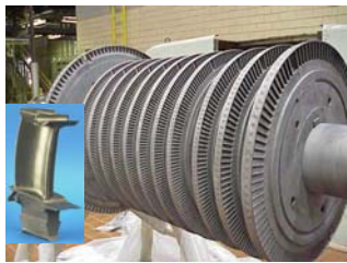
Fig. 3. A section of turbine blades can be coated using the solution plasma spray for enhanced properties
