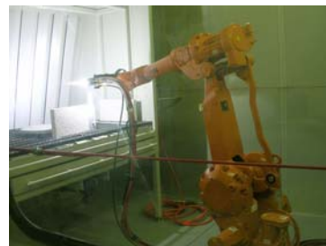
Fig. 1. The Plasma spraying technique in the process of making nanocomposite parts.
