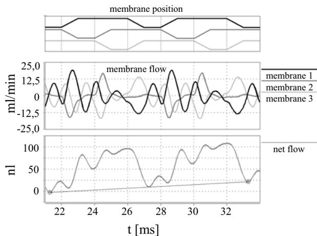
Figure 7: Driving profile and resulting flow characteristics for two pump cycles of a three-finger peristaltic pump.
