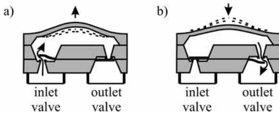
Figure 2: Flap-valve pump in a) supply and b) pump mode.
