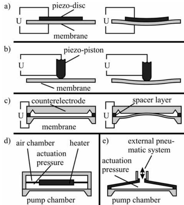
Figure 3: Different types of actuation principles [5]. Piezoelectric drives: a) piezo disc, b) piezo piston; c) electrostatic drive; d) thermopneumatic drive and e) pneumatic drive
