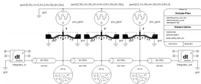
Figure 6: Setup for an peristaltic pump with the elements of the toolkit.
