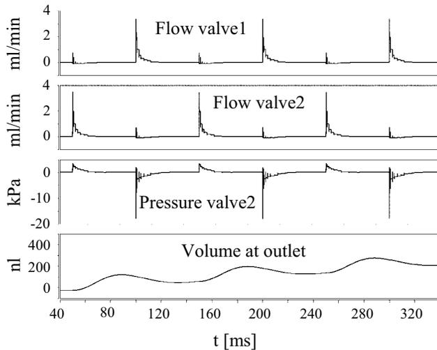
Figure 5: Results of the flow characteristics for a pneumatic actuation of the flap valve pump driven by a pump frequency of 10 Hz.
