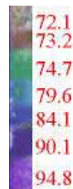
Figure 4: Lookup table of TLC of red starting at 92 ^{\circ} C and blue starting at 98 ^{\circ} C
