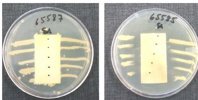
Figure 4. AATCC 147 test result against S. Aureus for a non-treated fabric sample as a reference (left) and for a silver salt treated fabric (right) exhibiting, respectively, no peripheral inhibition and a measurable zone of inhibition.
