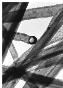
Figure 2: TEM image of an aluminum nanotube.
