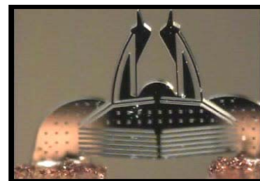
Figure 1: 50- \mu\text{m} thick, electrothermal microgripper.
