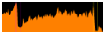
(b) The line profile of AFM in the length of 5µm. The maximum height of the rectangular is 3.47 nm.
