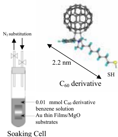
Figure 2: Schematic equipment of the SAM process and the used \text{C}_{60} derivative ( \text{C}_{60}\text{-O-C}_8\text{SH} ). The soaking cell was filled with \text{N}_2 gas. The soak was done at room temperature for 20 hr.
