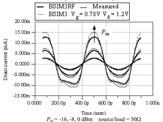
Figure 5: Time-domain waveform for output drain voltage
