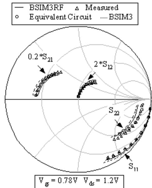
Figure 4: Comparison between the measured, BSIM3RF and equivalent circuit S-parameters
