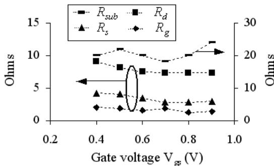
Figure 3:  $R_g$ ,  $R_d$ ,  $R_s$  and  $R_{sub}$  extracted data for  $V_d = 0.2V$
