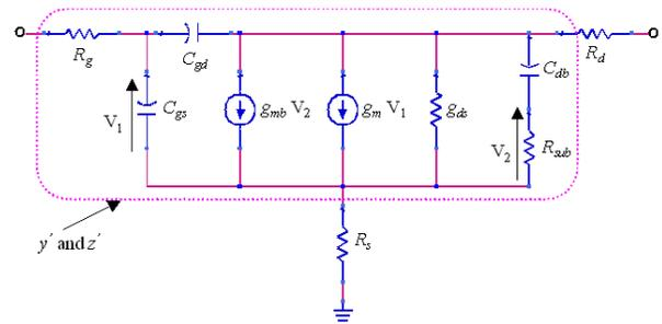
Figure 1: Small-signal equivalent circuit of a MOS transistor valid in all region of operation.
