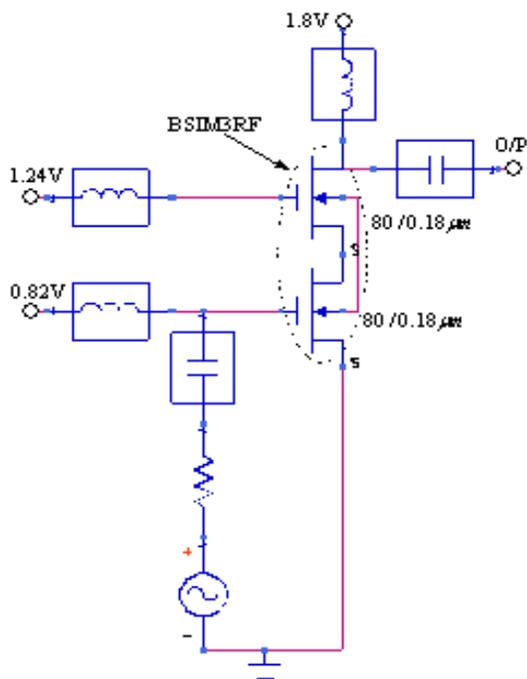
Figure 6: Schematic of CMOS power amplifier
