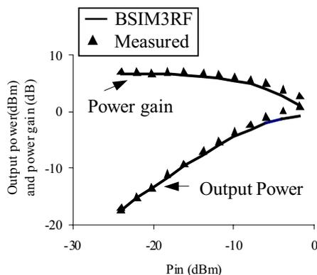
Figure 7: Fundamental power sweep source/load = 50Ω
