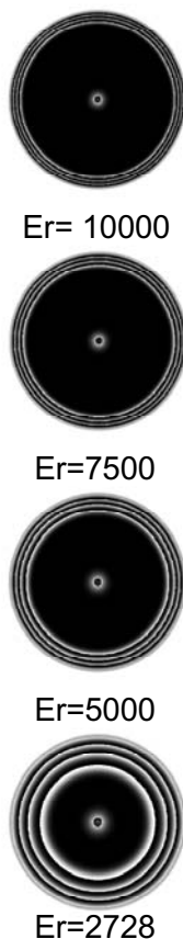
Figure 6: Texture simulation of the fiber cross section shown the average orientation to the secondary solution S_{+4} at Ericksen number 10000, 7500, 5000, and 2728.
