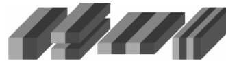
Figure 1: Schematic of a SAR step: initial configuration, splitting, recombination, reshaping (from left to right).
