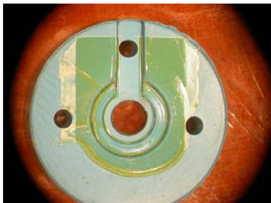
Figure 4: Green tape CIT structure with photolithography done.
