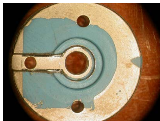
Figure 5: Green tape CIT structure plated with electro-less Ni.
