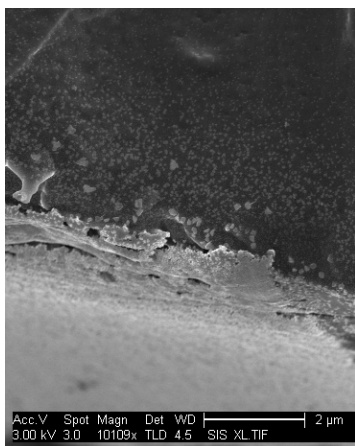
Figure 6: Au colloids assembled on Flemion sample 3 (cross section view), the cross linker is mercaptoethanol.
