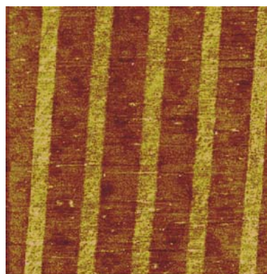
Figure 2. An AFM friction image ( 25 \times 25 \mu\text{m}^2 ) of a TBDMS SAM patterned by \mu CP with oxidized PDMS stamps (dark areas: TBDMS, bright areas: hydrolyzed TBDMS).
