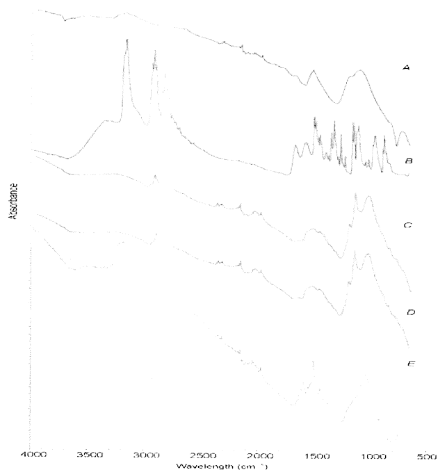
Figure 2. ATR-FTIR spectra of fluoronanotubes 1 (A), and functionalized SWNTs: 3a (B), 3b (C), 3c (D), 3d (E).
