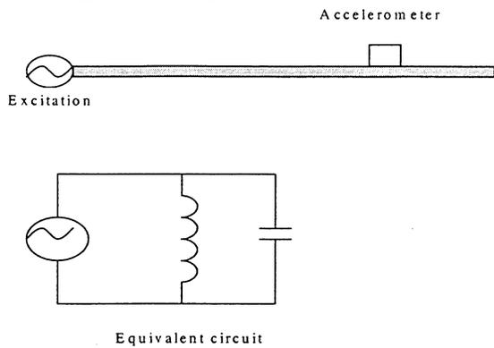
Figure 1: Beam model of structure under test, equivalent circuit and resonance
