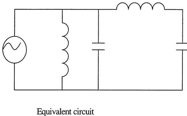
Figure 2: Detached accelerometer model and resonance
