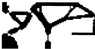
Figure 5: Gripper design with perpendicular constraint
