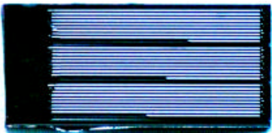
Figure 4: Micromachined meander network used for verifying models. Three menisci travelling through the channels at different positions.
