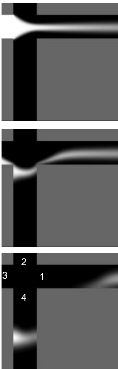
Figure 5. Pinched injection sequence: focusing step (top), injection (middle), separation (bottom).
