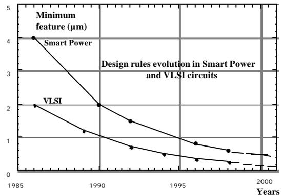
Figure 4: Evolution of minimum features in Ics and in Smart Power devices.
