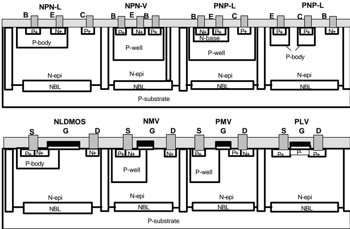
Figure 3: Schematic cross-sections of some important bipolar and MOS devices in power integrated devices mixing MOS and bipolar devices [8,9].
