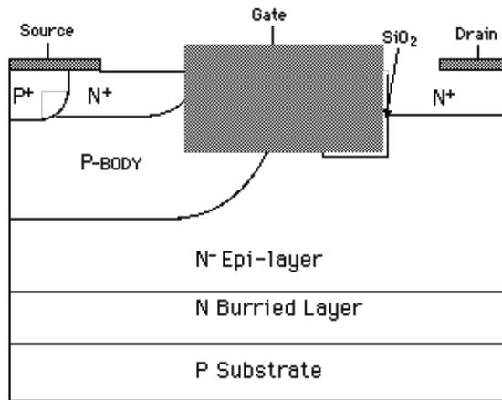
Figure 5: Schematic cross-section of a new LUDMOS device [17].
