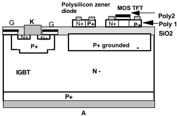
Figure 6: Schematic cross-section of discrete power device integrating protection functions [23].
