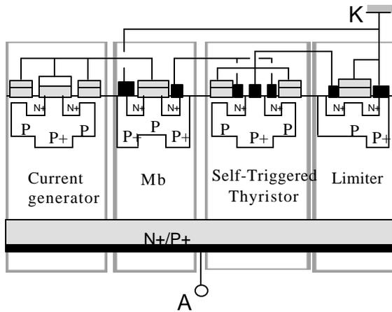
Figure 9: Cross sectional view of the integrated device.
