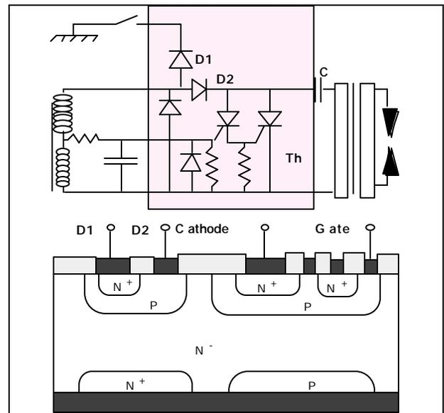
Figure 7: Programmable lightning protector for a subscriber line interface circuit by STM.
