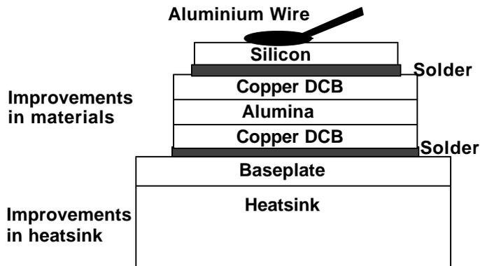
Figure 11: Schematic of conventional module assembly.
