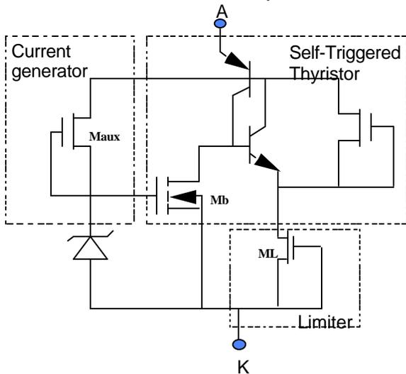
Figure 8: Equivalent electric circuit of the breaker-type protection function.
