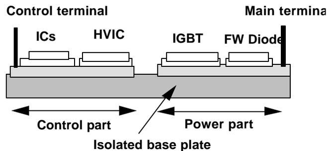
Figure 10: Schematic of ASIPM assembly.
