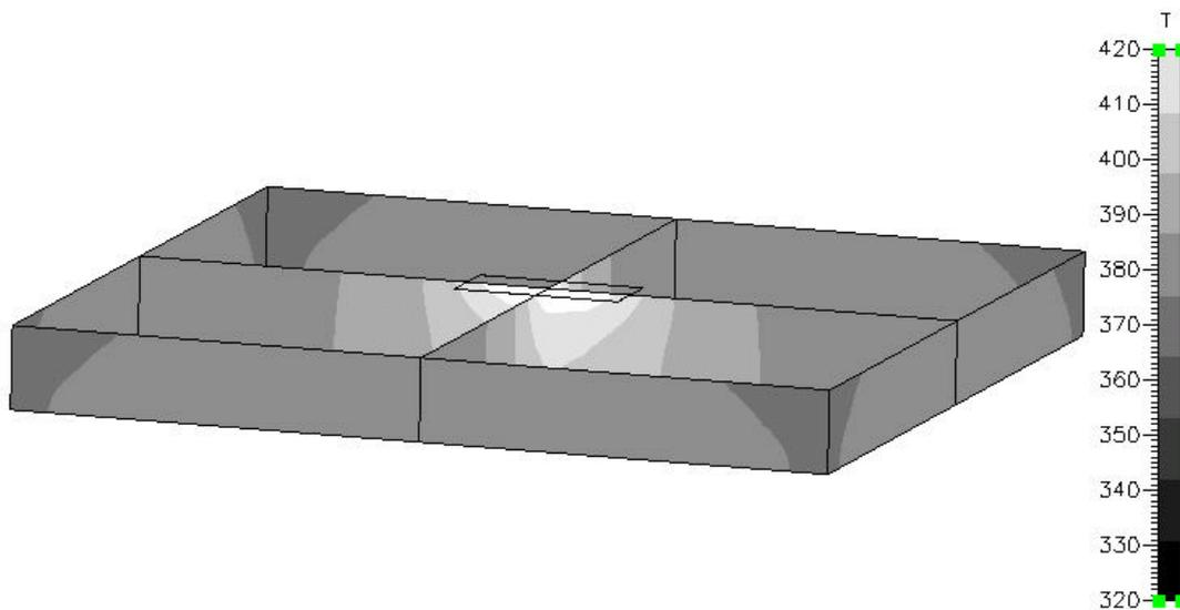
Fig. 3 Calculation of temperature distribution in the Si-chip, the small rectangle on the top represents the heated Pt-layer; heating power 10W; heating time 1 s
