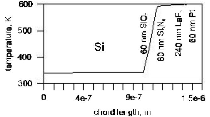
Fig. 6 Temperature profile for short electrical heating impulses; heating power 100 W; heating time 10  $\mu\text{s}$
