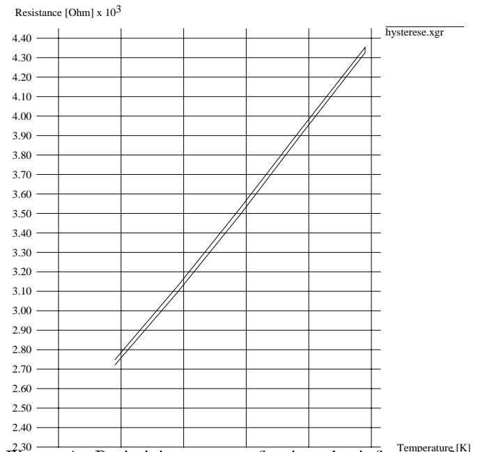
Figure 4: Resistivity curves reflecting the influence of thermo-mechanical loads on the embedded resistor. The mechanical simulation allowed for inelastic deformation.
