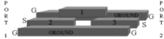
Figure 7: A resistive MEMS switch structure.
