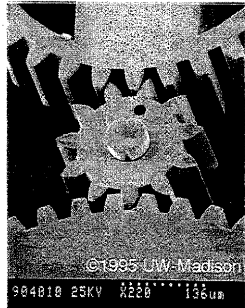
Figure 1: Example of a MEMS nickel gear train. Dimensions: approx. 200 microns. Courtesy Prof. H. Guckel, University of Wisconsin. [1]
