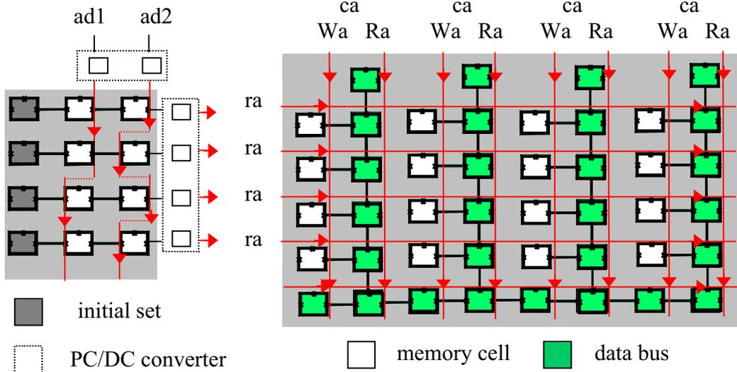
Fig.5 Josephson PC memory array with address decoder
