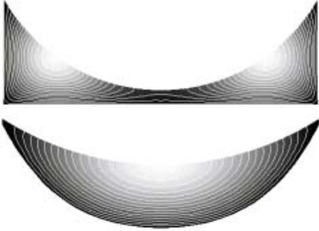
Figure 2: Flow velocity contours in EDM machined (above) and etched grooves (below). High velocities are indicated in light colors.
