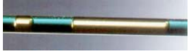
Fig. 2. Photograph of ferrofluid plugs separating reagents flowing in a capillary tube.
