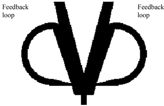
Figure 2: Typical feedback oscillator configuration derived from wall attachment fluidic amplifier.
