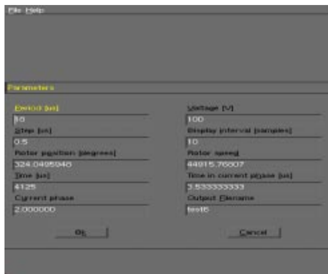
Figure 3: The dialog box allows changing the parameters of the micromotor dynamic simulation and initial conditions, as displayed by MICROTOR program.
