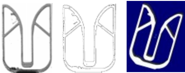
a) Original image b) Extracted edge c) 3-D model Figure 3: 3-D model reconstruction.
