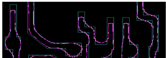
Figure 2: PRINTimage contour compared with intended design and full wafer image.
