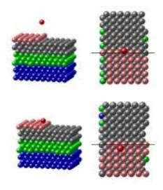
Figure 1: Sequence of snapshots (side and top views) of molecular dynamics simulations of deposition near a monatomic step showing effects of steering.
