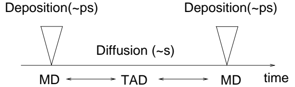
Figure 1: Standard MD allows one to simulate deposition, since few ps of simulation are sufficient to model the process. Diffusion between subsequent depositions, on the other hand, occur on the s time-scale. In order to reach this long time scale we use the TAD method.
