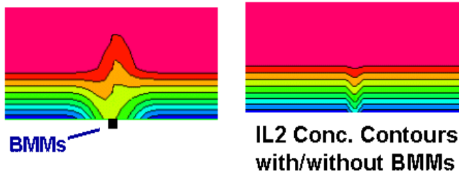
Figure 5: Bulk IL-2 concentration profiles at the end of the simulation. The upper figure is with the biomotors as an agitation device, the lower figure is without the biomotors.
