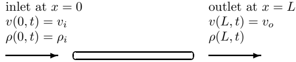
FIG. 1. Schematics of the flow configurations. The quantities v_i and \rho_i are, respectively, the inlet velocity and density while the outlet velocity is denoted by v_o .
