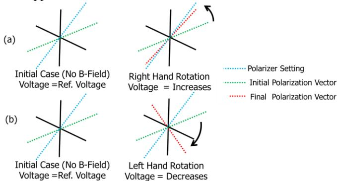
Figure 4: Correlating rotation to changes in intensity
