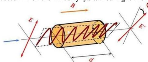
Figure 1: Rotation of polarized light during FR
