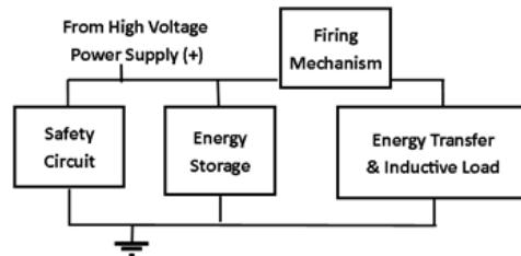
Figure 3: Block diagram of pulsed magnetic field circuit
