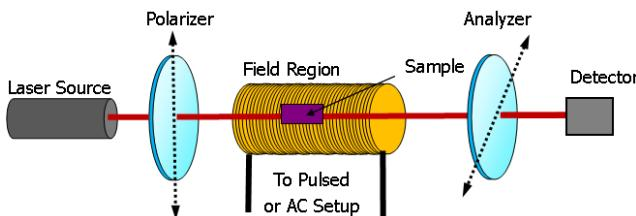
Figure 2: Important aspects of a FR experimental setup
