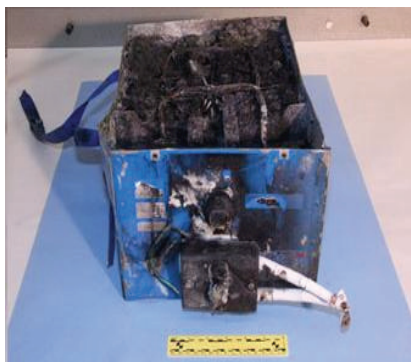
Fig. 2 ‘Dreamliner Jet’: Li-ion Battery exploded on-flight [14].
