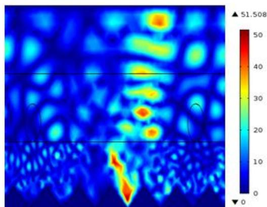
Figure 2: Electric field magnitude for elliptical nanoparticles interacting with a periodic back-reflector.
