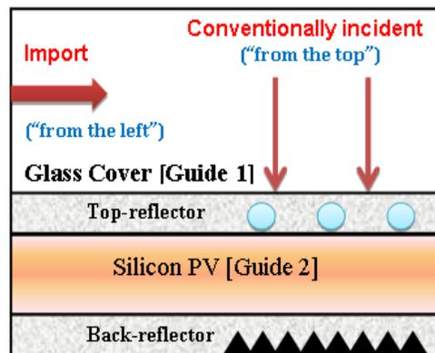
Figure 1: A mode trapping architecture.
