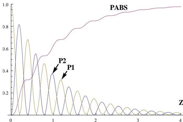
Figure 3: Rapid absorption in a linear light-trap.
