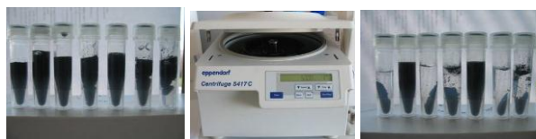
Fig. 2. Seven MWCNT-dispersions in water (left); centrifuge (middle); dispersions without or with suitable IL after 20000 rcf, 1 min (right).
