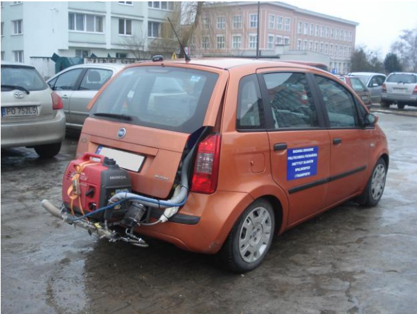
Figure 3: Vehicle with a mounted apparatus for measuring particle parameters.
