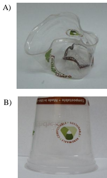
Figure 1: Image of poly(lactic acid) cups with a) low level and b) high level of crystallinity following the addition of boiling water. The highly crystalline cup was annealed at 110 °C for 10 min in order to induce a high level of crystallinity, thereby preventing distortion in the cup at high temperatures.
