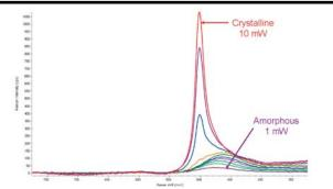
Figure 4: The effect of excitation laser power on amorphous silicon. The 532 nm excitation laser power at the sample was controlled by the DXR Raman microscope laser power regulator and was increased in 1 mW steps from 1 to 10 mW. Results show little effect on the amorphous silicon at power levels up to 4 mW. Higher laser power progressively converts the amorphous silicon to the crystalline form.
