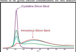
Figure 1: Raman spectra of silicon samples ranging from pure crystalline to predominantly amorphous silicon.
