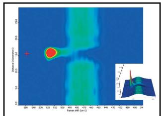
Figure 2: A 30 micron line map across a sample of deposited silicon. Raman intensity is indicated by color (high intensity is red; low intensity is blue).
