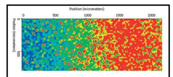
Figure 3: A  $750 \times 2,250$  micron, two-dimensional map of a sample of silicon deposited on glass. The chemical image was generated by calculating the ratios of the peak heights at 521 and 480 cm-1 at each point on the map. Crystalline areas are shown in red and amorphous in blue.
