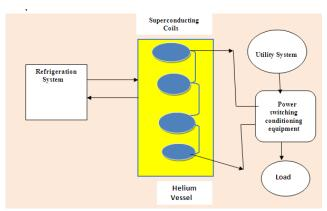
Fig 2: Operation of a superconducting magnetic energy storage system
