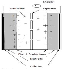
Fig 6 Ultracapacitors [10]
