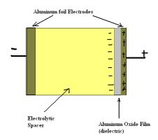
Fig 5 electrolytic capacitors [9]
