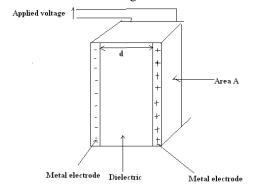
Figure 4: The principle of capacitors[8]
