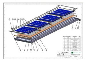
Figure 4: The combined MSS (PV/T) Collector
