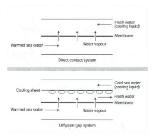
Figure 2: Membrane distillation (pervaporation) system
